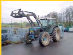
7840 SLE Bj. 1993 73 KW (100 PS) 8.200 h 4*DW, STOLL FL ROBUST F 30 HD - EURO SN: 5023145 BJ. 2001, AUTOM. AHK; PITON-FIX
